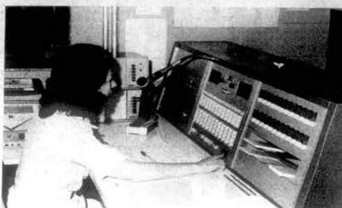
LOUDON JUSTICE CENTER Chief Communications Dispatcher Casey Lenex broadcasts a citizens complaint to a county sheriff's patrol car over the new communications system that has just been installed in the center. The versatile new system has many features including cross patching of frequencies and telephone patching into the radio system.
