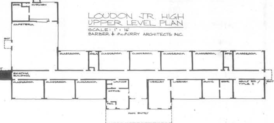
JUNIOR HIGH ADDITION —This architects drawing shows the proposed addition of a gymnasium-auditorium and five classrooms to Loudon Junior High School. The drawing (with new construction areas shaded) shows only four classrooms. The fifth is on the lower level. The proposed cost of the addition is over $750,000.
