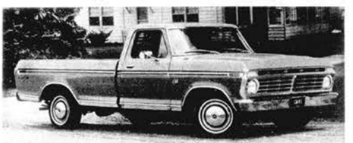
F-100 PICKUP TRUCK—Ford Division's new F-Series pickup trucks, including this F-100 Ranger XLT, feature the most extensive changes in six years. The F-100 250-300 light trucks include an all-new cab, new interiors, new exterior sheet metal, longer wheelbases and wider tracks. Cab length is increased two inches, permitting more leg room and a roomy storage area behind the seat in most models. New features include front disc brakes on all two-wheel-drive models, double wall construction of the cargo box and optional power steering and automatic transmission in four-wheel-drive models.
